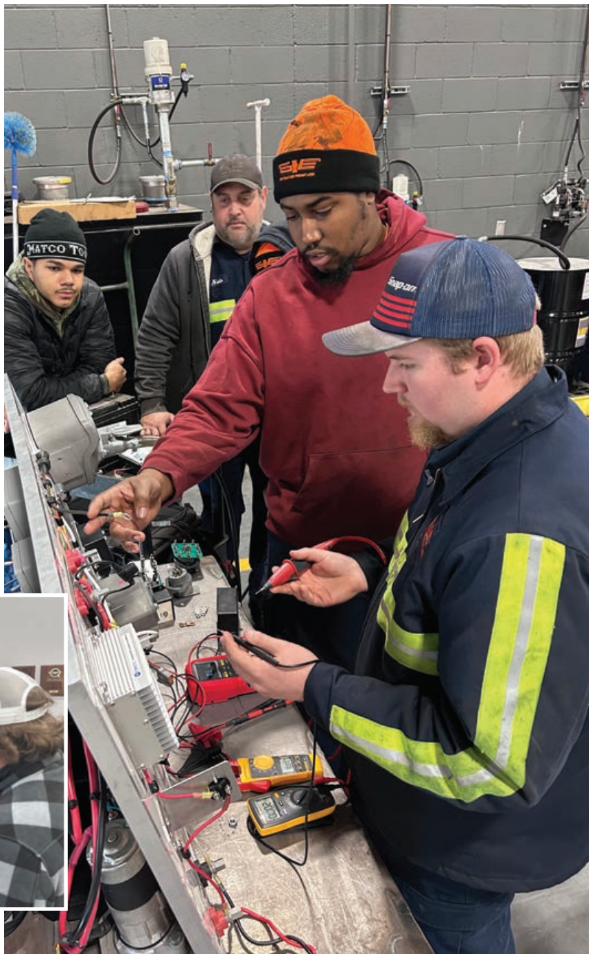
Josh Bell (West Atlanta) and Brett Smith (Dalton) work to diagnose a liftgate charging system
